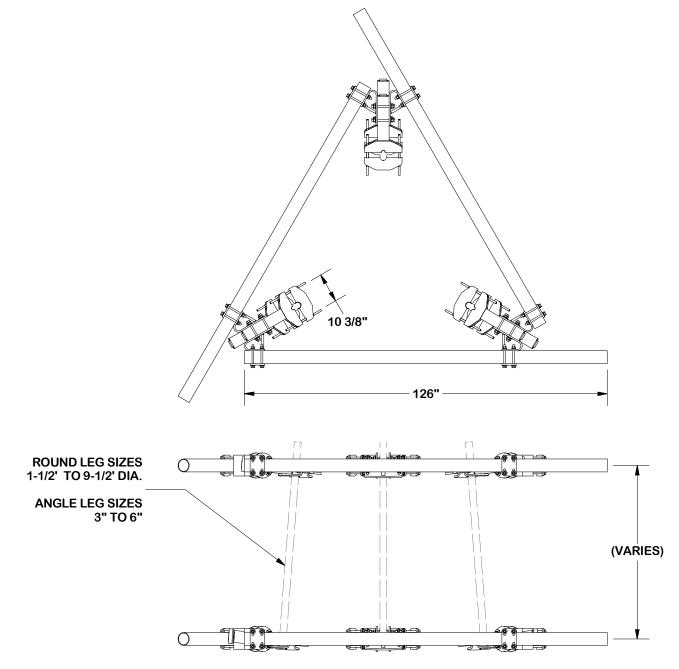
**TAPER NOTE:** THE MAXIMUM TAPER ADJUSTMENT IS 8° BASED UPON 60" SPACING OF ADJUSTABLE MOUNTING BRACKETS.
